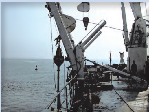
Box 3–1, Figure 4. Core apparatus located on the Marion Dufresne , used to take cores from Middle Tampa Bay. Photo from Edgar (2002).
